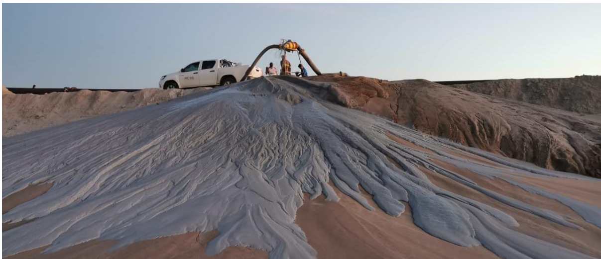
Figure 15: Example of cyclone deposition (source: international mining)
