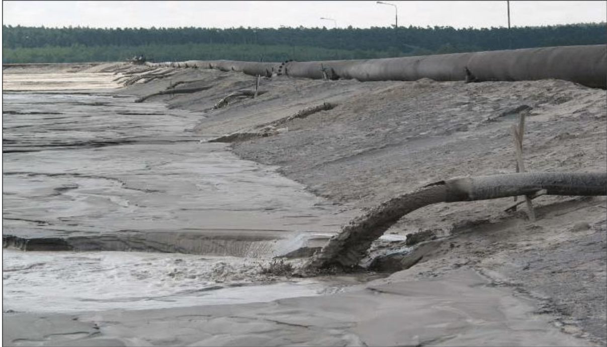
Figure 13: Example of spigot deposition (source: www.researchgate.net )
