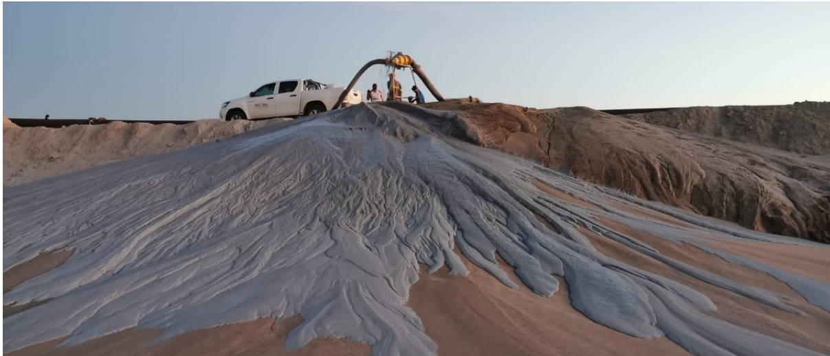
Figure 30: Example of cyclone deposition (source: international mining)
