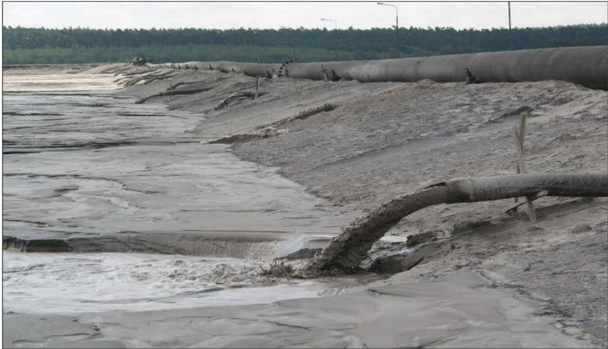
Figure 28: Example of spigot deposition (source: www.researchgate.net )
