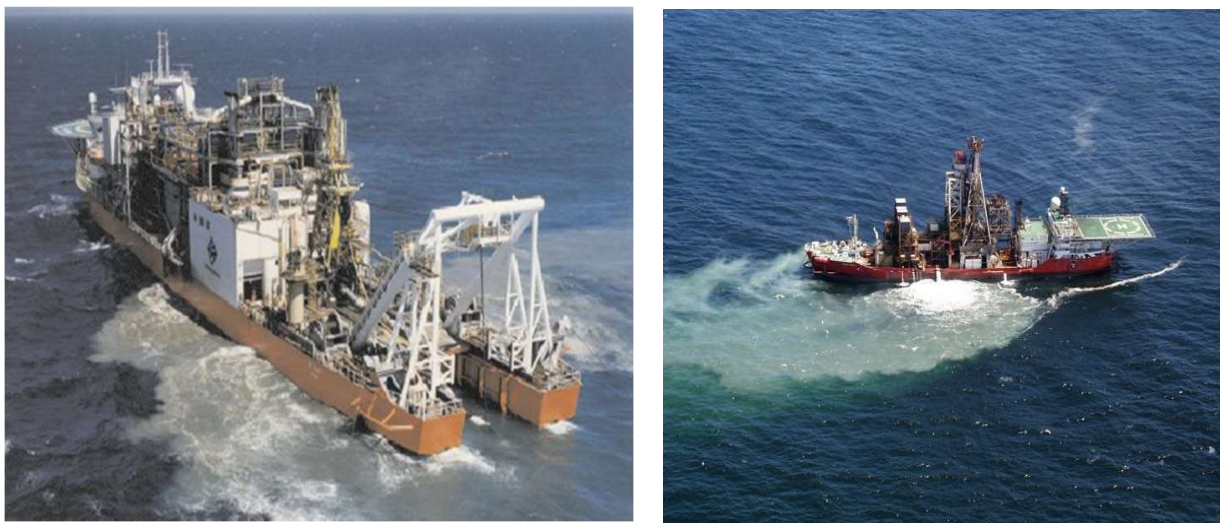
Figure 143: Typical crawler-vessel (left) and drillship (right) operating in the Atlantic 1 Mining Licence Area (Photos: De Beers Marine).
