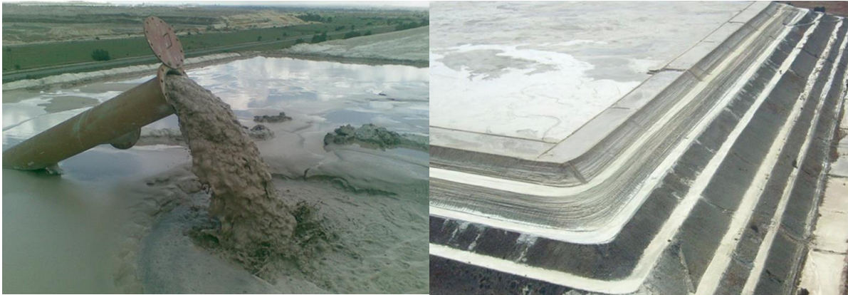
Figure 14: Example of daywall deposition. An open-ended discharge at one end of the paddock daywall (left) and small impoundments with dried-out tailings (right) (Goldfields, 2023)
