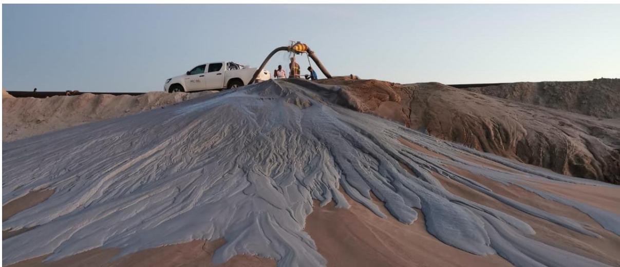
Figure 8: Example of cyclone deposition
