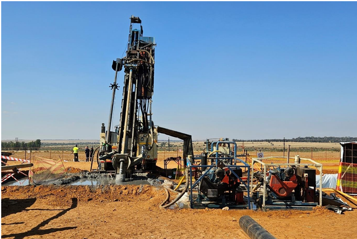
Figure 7: Example of a typical drill rig used during exploration drilling.
