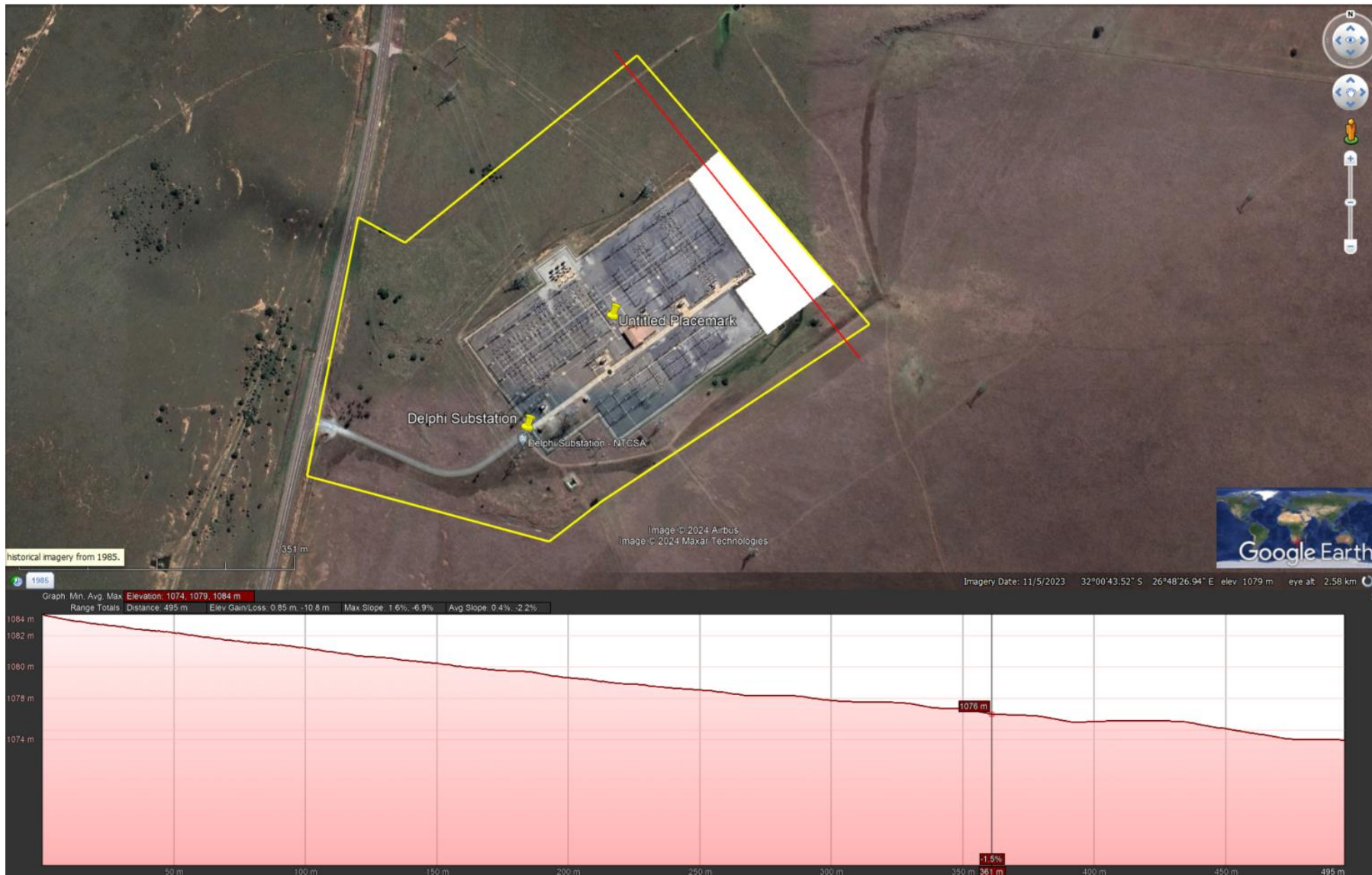
Figure 9: Elevation profile of the NTCSA Delphi Substation Expansion site.
