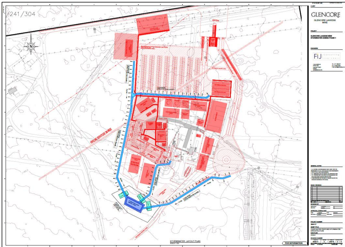
Figure 3-1 Proposed stormwater design for the proposed development (FIJ Consulting Engineers, 2025)
