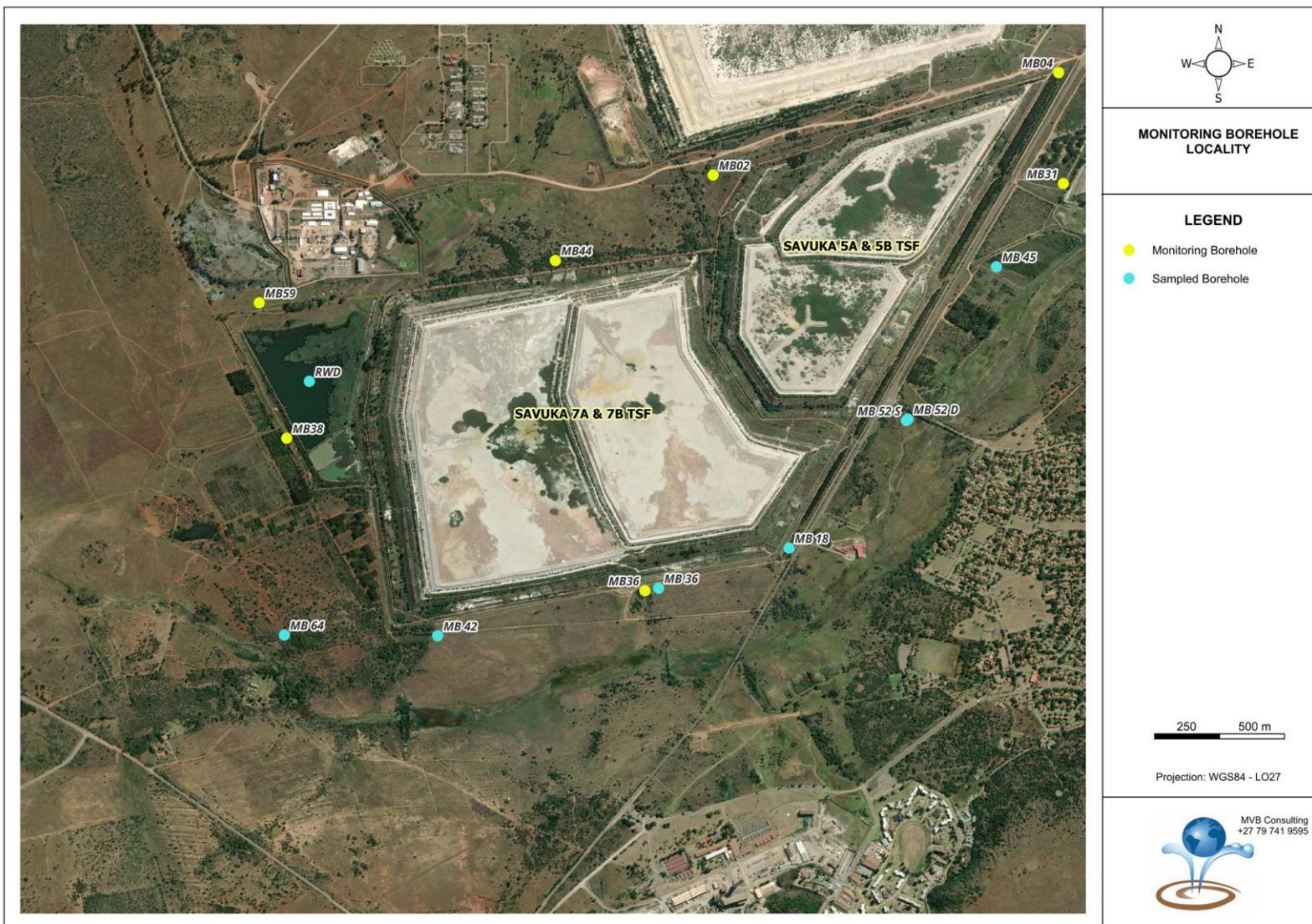
Figure 22: Monitoring Boreholes Locations
