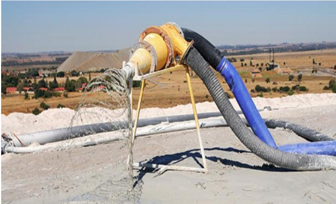
Figure 44: Example of cyclone deposition (Goldfields, 2023).
