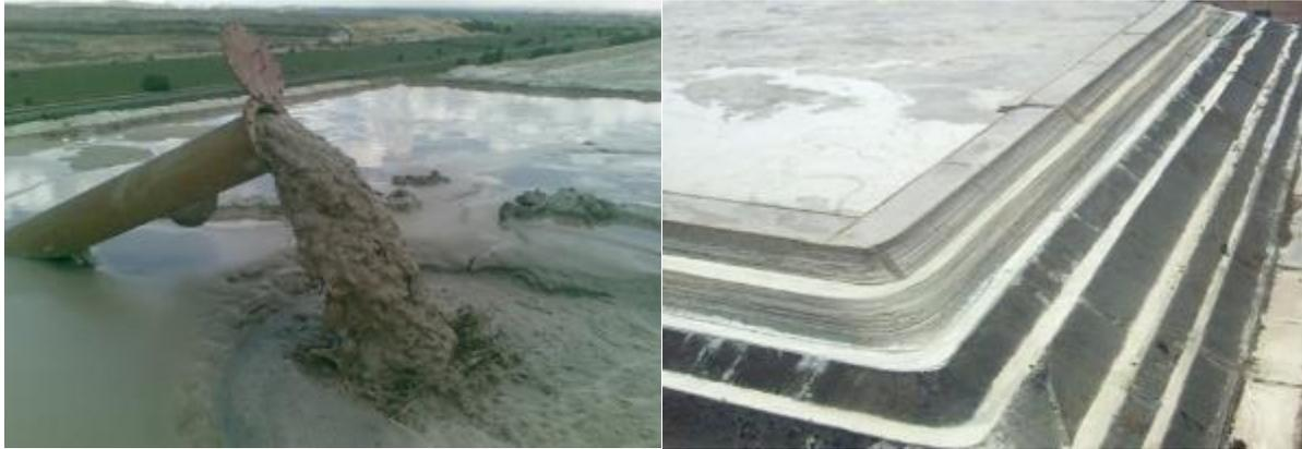
Figure 43: Example of daywall deposition. An open-ended discharge at one end of the paddock daywall (left) and small impoundments with dried-out tailings (right) (Goldfields, 2023).
