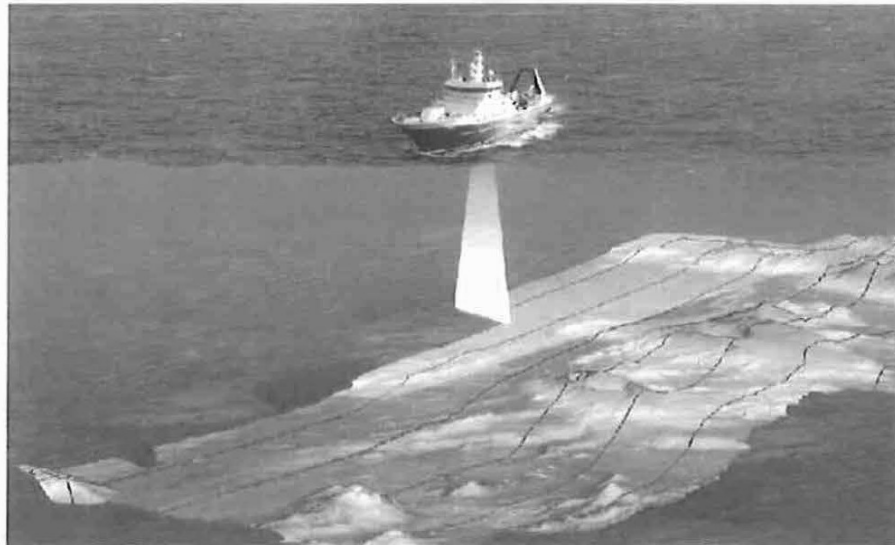
Figure 2: Schematic of a vessel using multi-beam depth/echo sounders ( http://www.gns.cri.nz/ ).
