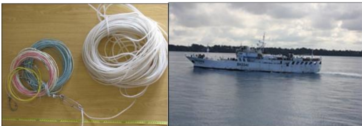
Figure 47: Photograph of a mainline (braided monofilament) with a dropper line and trace typically used by the pelagic long-line fishery (white line) (Left) and a typical high seas longliner active in South African water (Right) (CapFish, 2014).
