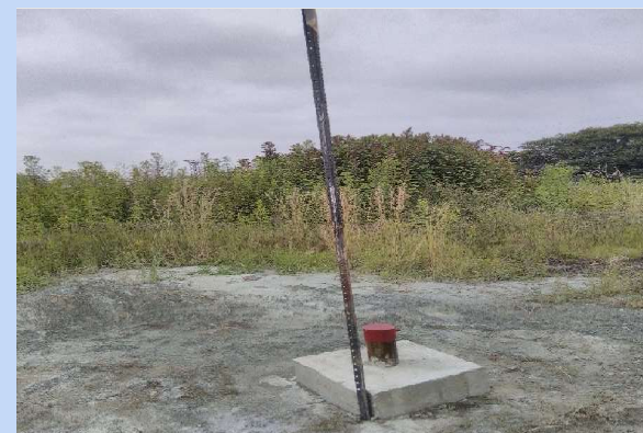
Newly drilled monitoring borehole - Mar 2025
