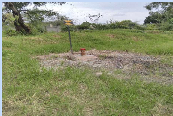
Newly drilled monitoring borehole - Mar 2025
