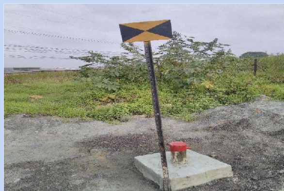
Newly drilled monitoring borehole - Mar 2025
