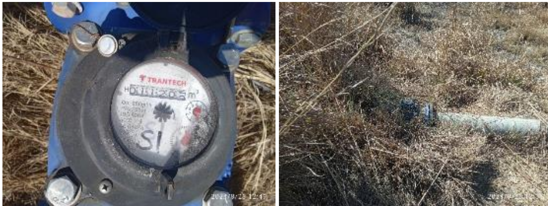
Figure 5: Flow meters observed in a good condition. The readings are recorded by the mine staff.
