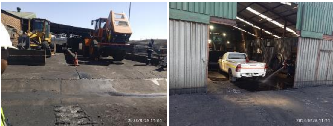
Figure 10: View of workshop impervious surface and drainage and car washing activity with potential to pollute the environment
